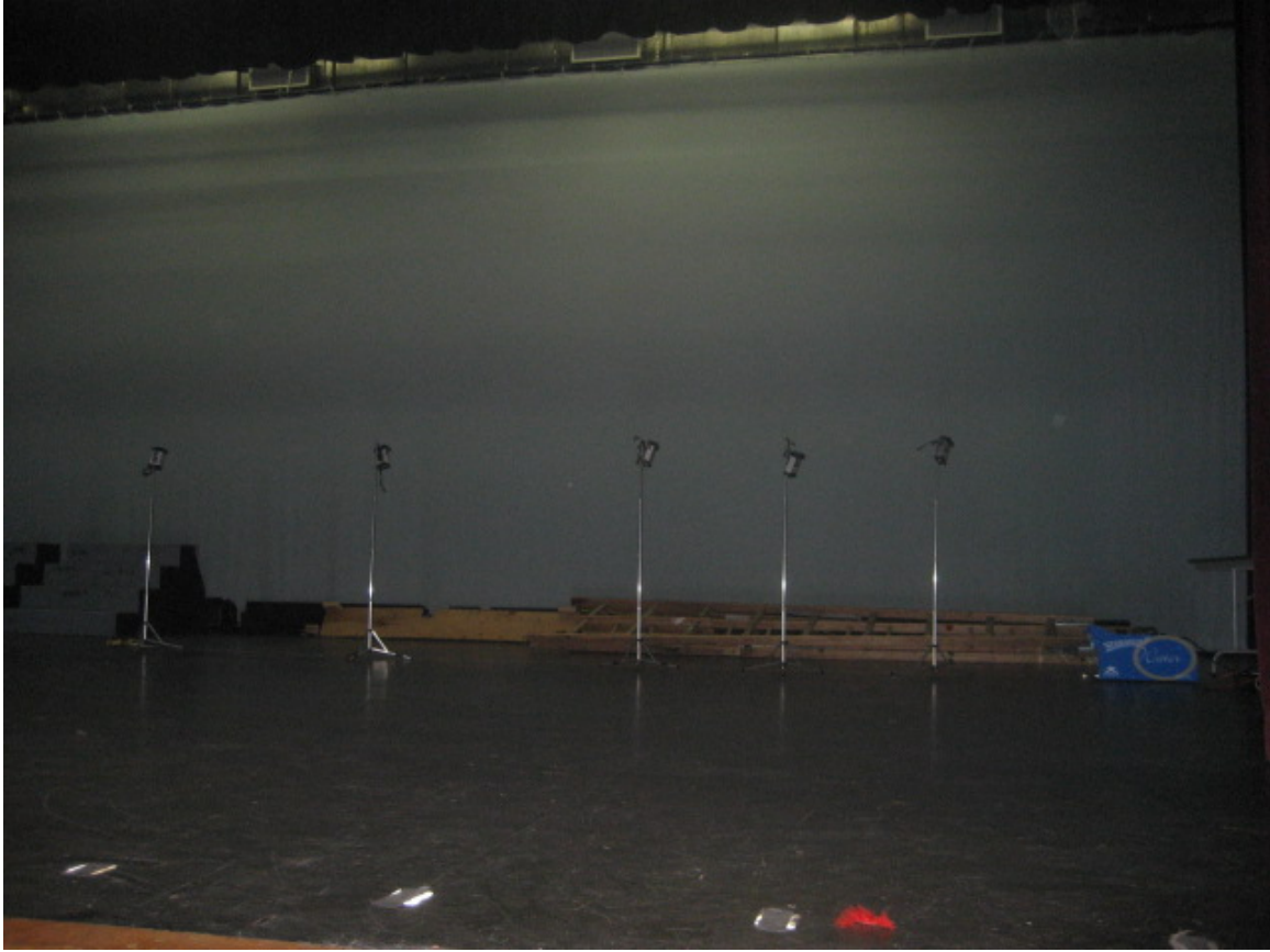
Figure 2. Monitoring configuration consisting of five tripod-mounted aerosol monitors situated at three-foot intervals from the Starhazer III machine. Each tripod is equipped with an aerosol monitor.
